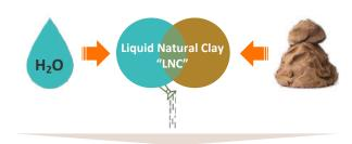
Liquid is applied onto the surface, and percolates down to form a soil structure that retains water like a sponge
